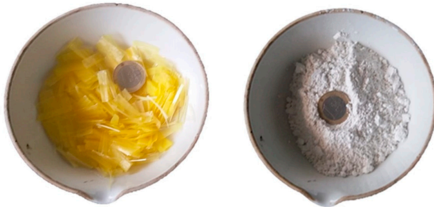
Figure 1. Modifiers used in this research. Pol-Aram fibers (left) and hydrated lime (right).
