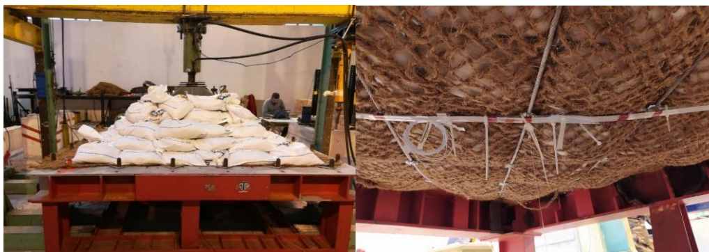
Figure 86. a) Distributed load test where the fiber Bragg grating monitoring was tested, b) plate with glued fiber bragg along the diagonal cable of the membrane
