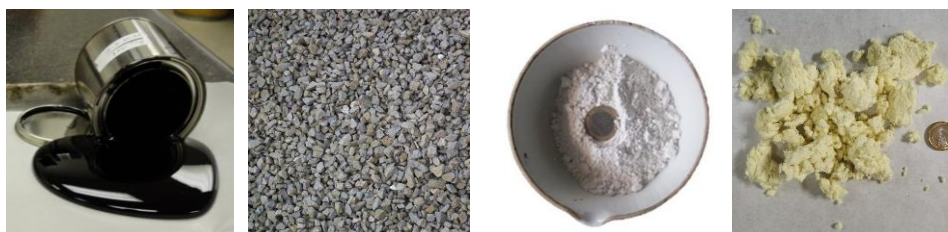
Figure 87. Materials of experimental mixtures (from left to right): polymer-modified bitumen, natural aggregates, hydrated lime and aramid fibres
